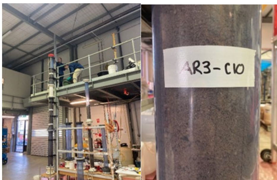
Figure 3: ANSTO Facilities, Column C10 at 4m height, and displaying positive agglomeration and 'heaping' characteristics
